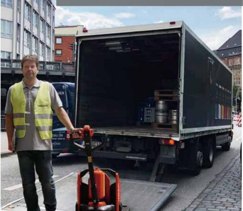
The function of driving with tiller in the **vertical position** helps with work in confined areas, especially in elevators and lorries without
