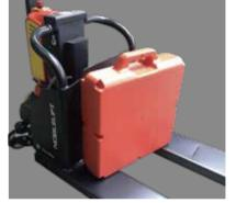
The PTE 20B truck is equipped with maintenance-free AGM battery pack, the charging time is 8 hours, opportunity charging is not available.
