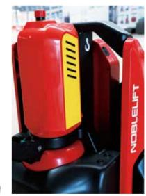
For the pallet trucks there are no hoses or pipes used in the hydraulic lifting circuit which significantly improves **reliability** and reduces the amount of potential problems related to leakages through connectors or their seals.
