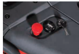
Key-switch, emergency switch and battery discharge indicator.
