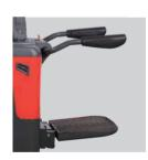
Optional foldable platform with protective arms. The cushioned platforms ensure safety in all travelling conditions.
